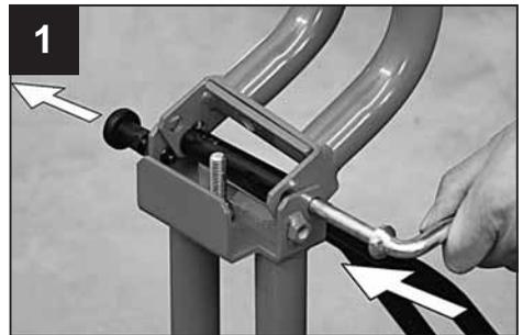
Insert all the different parts in the order shown in Fig. 2, then lock everything in place using the 22 mm hexagon spanner provided.
